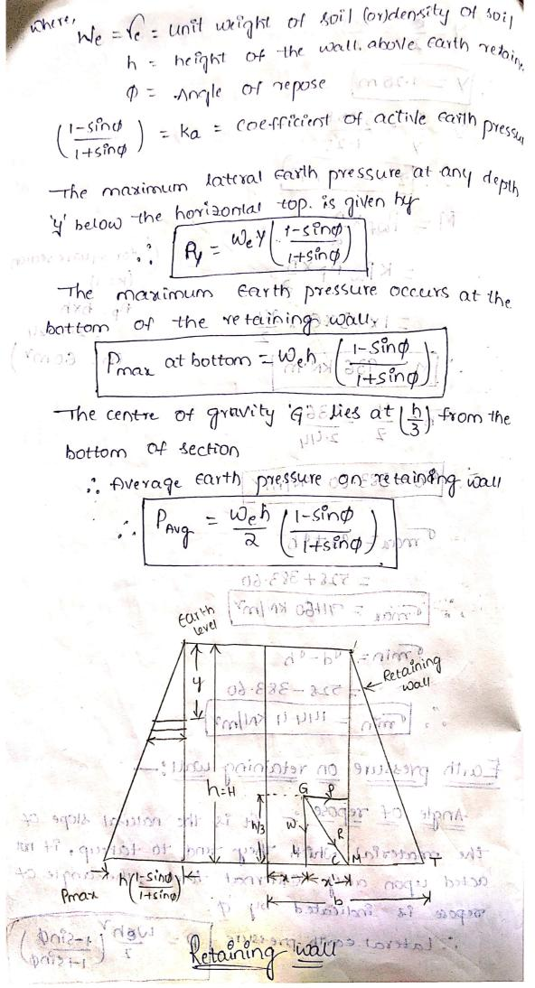
is 10m height and ereteins Earth which is level upto the top. The width at top is 2m and bottom is 8m the Exposed face is Vertical. Find the max. and min stress intensities at the base. Take deningly of Carth (We)(or) (Ve)=16kH/m<sup>3</sup>. density of masoning 24kH/m<sup>3</sup>. The angle of repose \$\phi=30^{\circ}\$
